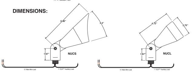
**FLEX**TM Unique Lighting Systems® fixtures are compatible with *FLEX*™ Series LEDs. Series LED lamps can be ordered separately.
